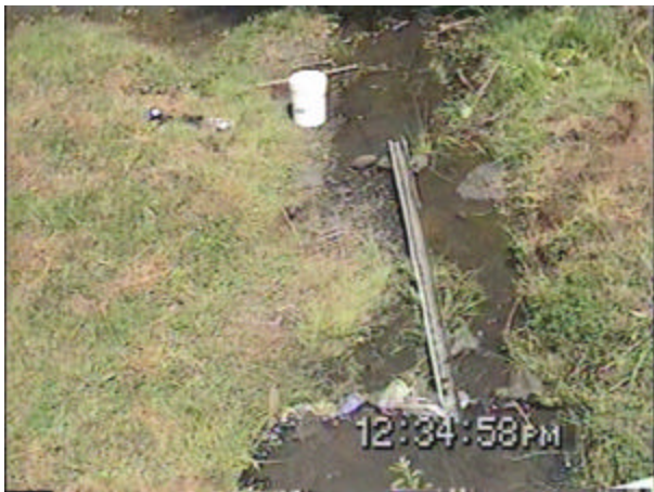
Figure 7 Flume used to measure the flow, which was 0.18 \text{ ft}^3 per second. The view is the downstream side at Wilson Rd. The stream was blocked and allowed to backfill. A hole was dug at the downstream end of the flume to accept the bucket. A stopwatch was used to time the filling of the bucket.
