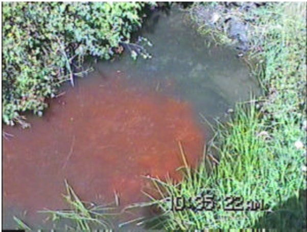
Figure 2 Leading edge of dye as it moves downstream near the injection point.
